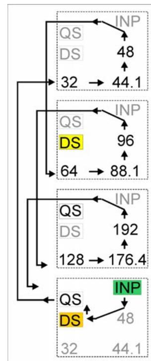
In case of SPDIF the incoming signal defines the status DS and QS. A manual selection is only necessary with ADAT. If an ADAT input signal is present, CLOCK also runs through DIG IN DS and DIG IN QS after DIG IN (INP).
