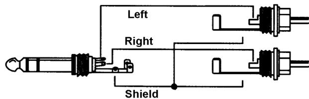
The pin assignment follows international standards. The left channel is connected to the tip, the right channel to the ring of the TRS jack/plug.
