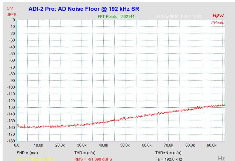
Indeed the rise in noise over frequency is much lower than in former converter chips, where for example at 192 kHz sample rate the wideband noise measurement would not reach -92 dBFS, but only -79 dBFS.
