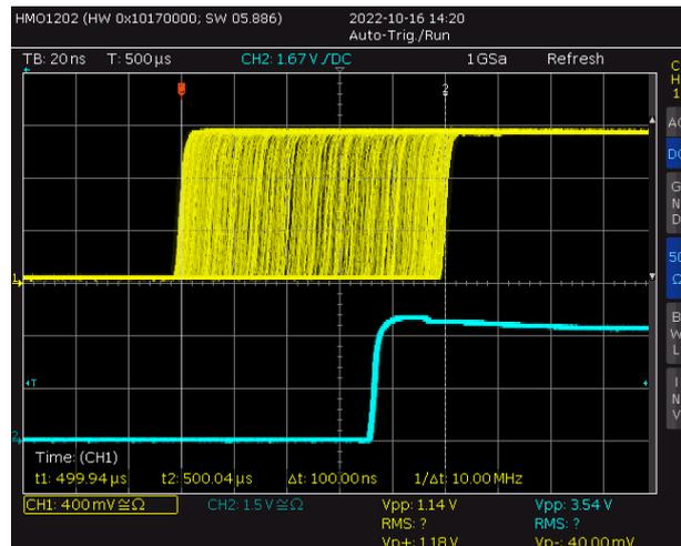
The so-called *sampling jitter*, usually in the range of picoseconds, is also very low in the ADI-2/4 Pro SE. Also remarkable is the identical performance when using internal or external clock – a typical SteadyClock feature. Check RME's YouTube channel for a video showing and explaining such measurements.
