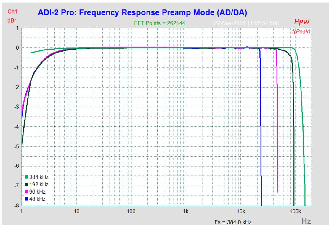
Note: 44.1 kHz to 192 kHz measured with filter Sharp on AD and DA..
