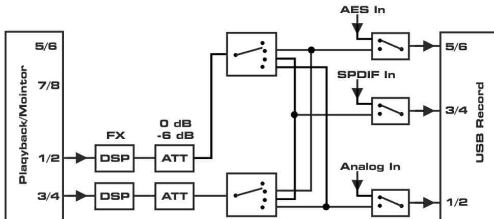
The simplified block diagram illustrates how the analog channels 1/2 and 3/4 are taken after the DSP FX processing (but before Volume, not shown) and routed to the USB recording channels 1 to 6. The original source (analog and digital inputs) is no longer present on the USB record path.
