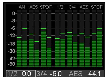
OVR appears for the rear XLR and TRS outputs at +2.5 dBFS, since the ADI-2 Pro FS R has this digital headroom. For the Phones outputs, OVR appears from +1 dBFS, since their analog circuitry limits the headroom here. In the horizontal meters of the EQ and Analyzer, the current peak hold value is displayed numerically on the right. Levels below -119 dB appear as UFL (Underflow).
