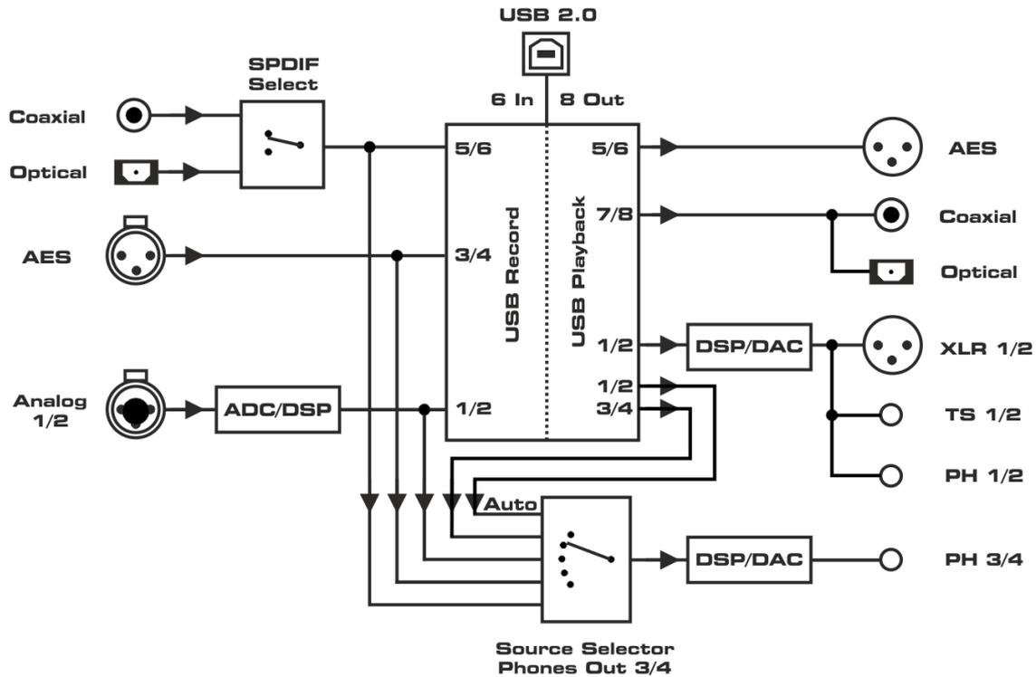
The option *Digital Out Source - Main Out* (SETUP – Options – Device Mode / DSD) sends the processed signal Main Out 1/2 also to the digital outputs AES, SPDIF and ADAT, for example to connect active monitors having digital inputs (not shown). The playback channels 5/6 and 7/8 can not be used anymore.
