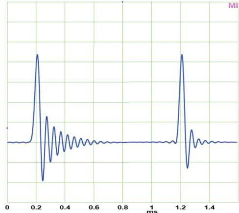
SD Sharp and SD Slow are IIR filters (also called minimum phase), which are not phase-linear and mostly cause post ringing. The advantage of IIR is the very low latency of a few samples only, which is welcome in a studio monitoring situation.
