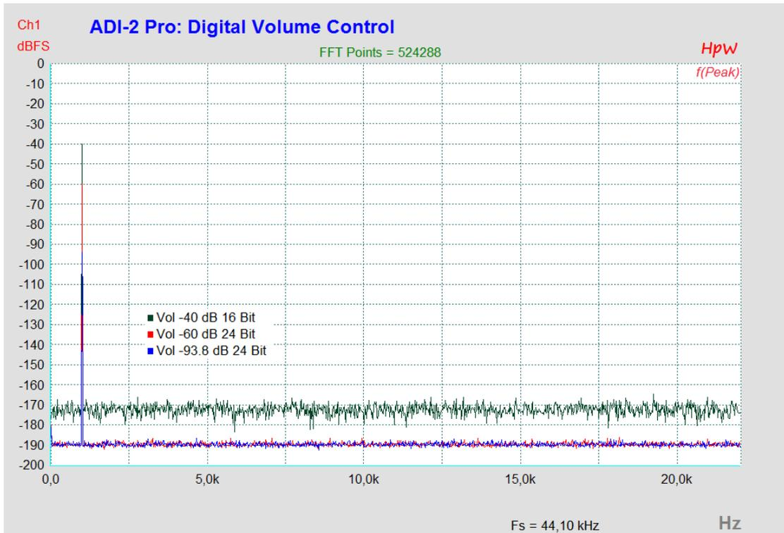
These results clearly show that distortion products of the digital volume control are not drowned by the DAC's noise, but are not generated at all. It works perfectly even with an undithered 16 bit signal, no detectable distortion products are produced.
