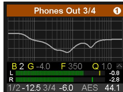
Pushing the EQ key a second time brings up the **EQ Enable / Presets** screen. In this screen the EQ can be switched on and off, and EQ presets can be stored and loaded comfortably.
