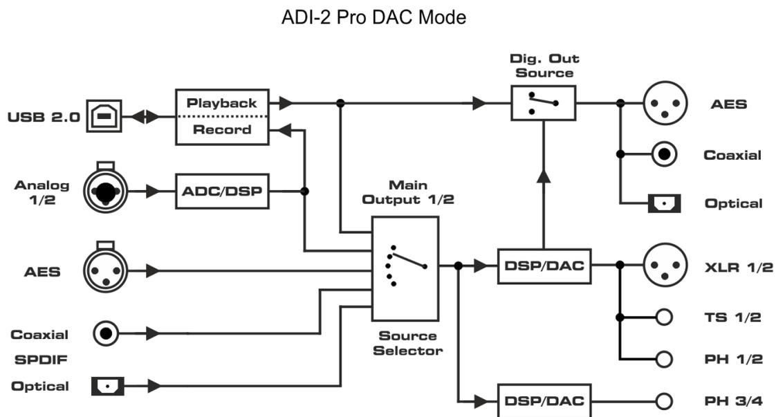
The option *Digital Out Source - Main Out* (SETUP – Options – Device Mode / DSD) sends the processed signal Main Out 1/2 also to the digital outputs AES, SPDIF and ADAT, for example to connect active monitors having digital inputs.
