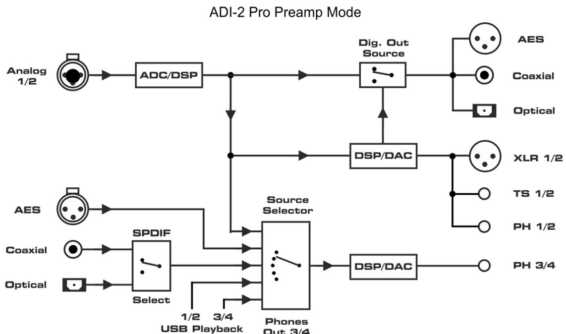
Note: To simplify the diagram and to maintain overview USB record is not shown. In all modes all input signals are sent over USB to the host. In multi-channel mode three separate stereo pairs, in stereo mode only the stereo analog input.
