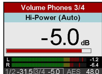
With revised volume settings, where the level meter stays below the red area, the user can now be 100% sure that the ADI-2 Pro operates absolutely free of distortion, even in the most extreme applications.
