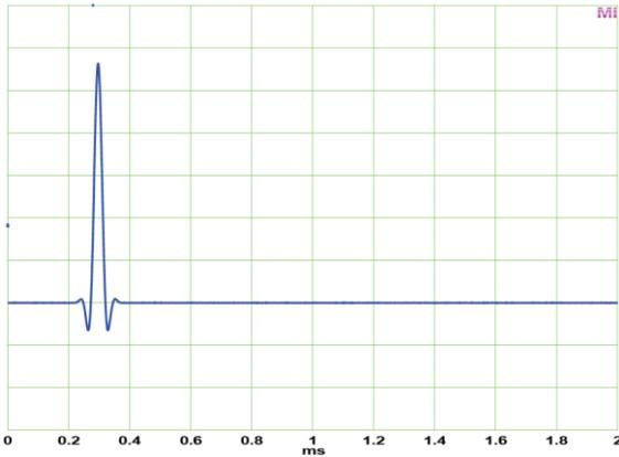
The screenshots above show the analog output signal of the DAC filters, stimulated by a digital single sample impulse at 44.1 kHz sample rate. While Slow has the most perfect response, it loses around 1.2 dB already at 15 kHz, see chapter 34.14. Both Short Delay are IIR filters, the other two are FIR type. FIR is phase linear over the whole frequency range.
