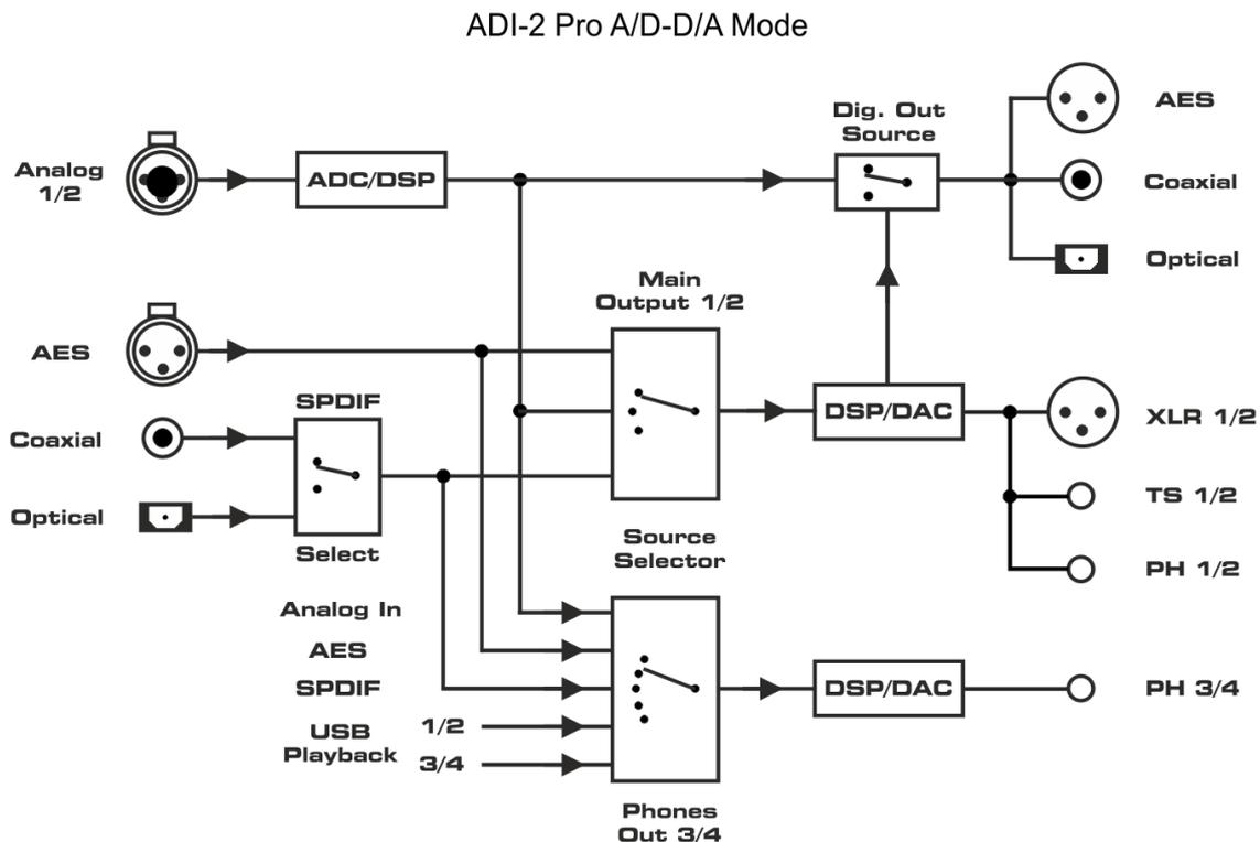
**Note:** To simplify the diagram and to maintain overview USB record is not shown. In all modes all input signals are sent over USB to the host. In multi-channel mode three separate stereo pairs, in stereo mode only the stereo analog input.
