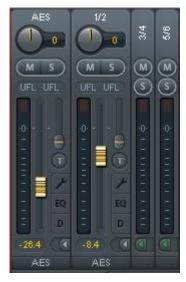
The **arrow symbol** at the bottom minimizes the channel width to that of the level meters. Another click maximizes it again. A mouse click with held Ctrl key causes all channels to the right to enlarge and minimize at once.
