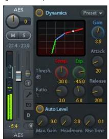
**Release.** Defines the release time for the control voltage of Compressor and Expander. Adjustable from 100 ms to 999 ms.
