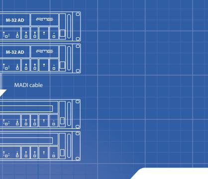
The AES3 and ADAT Routers and Converters make this type of setup simple and convenient - the twisted pair cable not only carries a bidirectional MADI signal, but also DC power on the same cable. Therefore, only the Routers have to be connected to a power source - the Converters receive their power via MADI TP.
